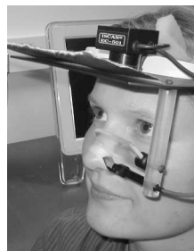
Figure 4. An ISCAN, Inc. headband-mounted eyetracker, set up for recording movement of the left eye during natural interactive task performance. Under the brim of the headband, an emitter sends infrared light down to the silvered mirror, which reflects it into the eye. Then the light bounces back and up to the eye camera, adjacent to the emitter, providing an image of the eye like that in Figure 3. The black cylinder underneath the silvered mirror is the scene camera whose image of the participant's field of view is reflected off the outside portion of the silvered mirror, off another mirror, and then into its lens.
