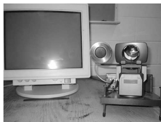
Figure 2. An ISCAN, Inc. remote video-based eyetracker, set up for recording movements of one or the other eye during viewing of simple scenes on a computer screen. The cylinder in between the monitor and the camera lens is the infrared emitter. The mechanism immediately below the camera itself allows it to tilt up and down and pan left and right to accommodate small head movements.
