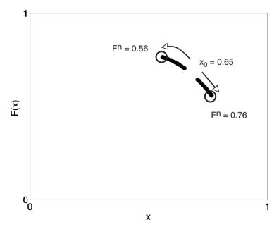
Figure 2. In this 'phase flow' diagram, the logistic map moves into two stable attractors with  $\mu = 3.1$ . The system starts at  $x_0 = 0.65$ . As the x is iterated through F, it settles into two attractor states, approximately 0.56 and 0.76, between which it will alternate indefinitely.
